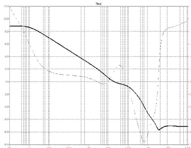
**Fig. 18. AC Simulation plot for 3 stage CMOS operational amplifier.**
