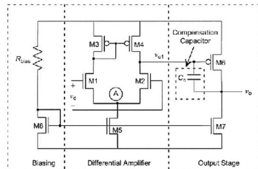
Fig. 1. Basic two stage operational amplifier.
