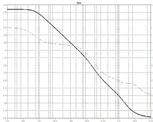
Fig. 10. AC Simulation plot for topology 1 , 2 stage CMOS operational amplifier.
