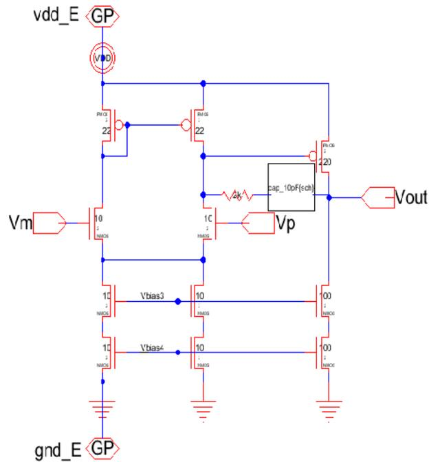
Fig. 4. Schematic for topology 2, 2 stage operational amplifier.
