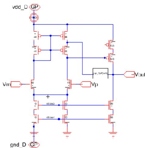
Fig. 5. Schematic for topology 3, two stage operational amplifier.
