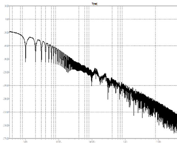
Fig. 11. FFT Analysis plot for topology 1, 2 stage CMOS Operational Amplifier.
