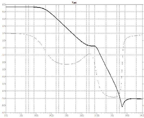
**Fig. 16.** AC Simulation plot for for topology 4, 2 stage CMOS operational amplifier.
