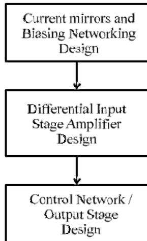
Fig. 8. Design Flow used for OpAmp Design.
