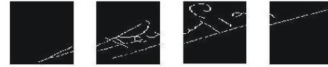
Image is partitioned in to four parts using equal horizontal density approximation method
