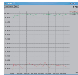
Fig. 3. Shows that the comparative packet delivery ratio between ack and modified ack.
