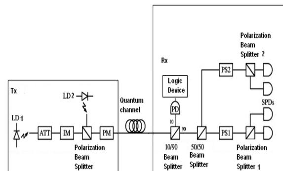
Fig. 1. Schematic of Quantum Key Distribution.
