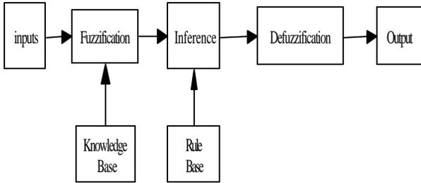
Fig. 1. Block diagram of typical fuzzy logic system and the general inference process.
