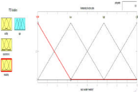
Fig. 5. FIS editor showing membership function plot of resistivity.
