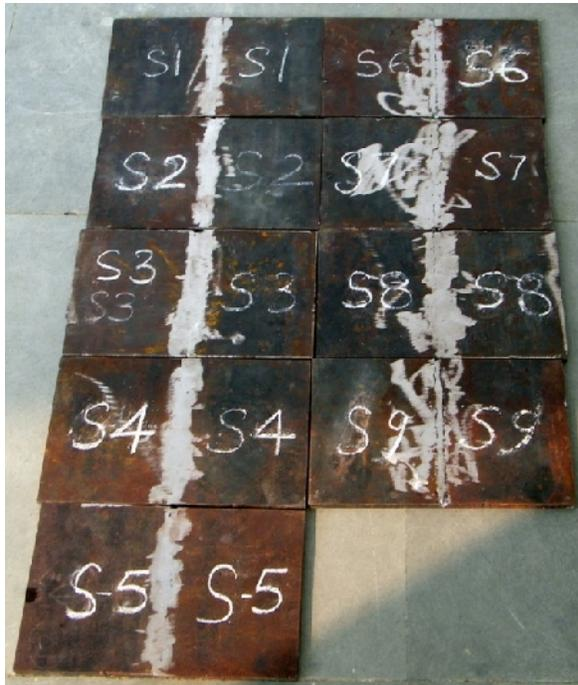
Fig. 2. Sample No. 1-9 after reinforcement grinding.
