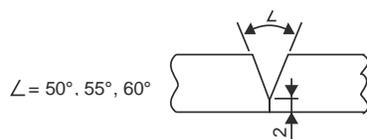
**Fig. 1. Preparation of Single 'V' Groove.**
