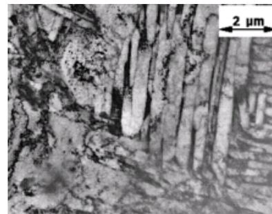
Fig. 2. Martensite Microstructure.
