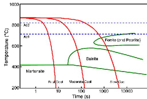
Fig. 1. Phase transformation in Austempering Process.
