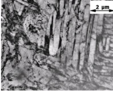
Fig. 3. Bainite Microstructure.
