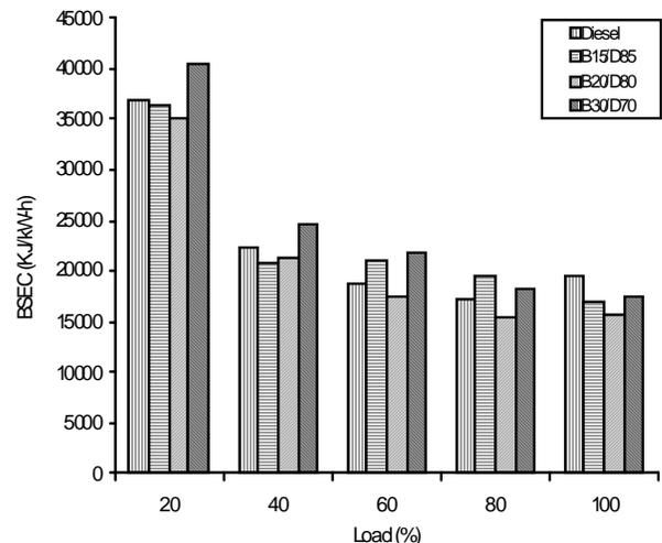
Fig. 4. Brake specific energy consumption Vs load.
