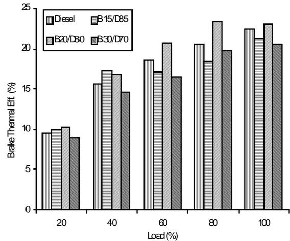
Fig. 3. Brake thermal efficiency Vs load.
