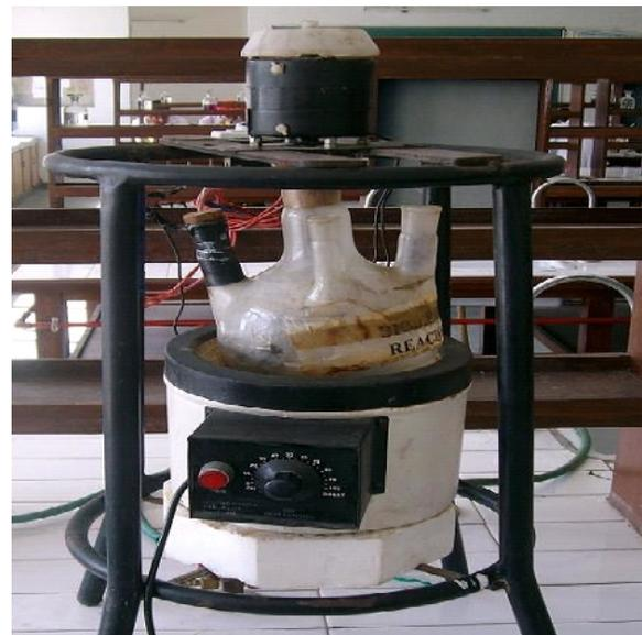
Fig. 1. Biodiesel reactor 2L capacity.
