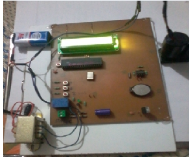
Fig. 6. Snapshot of Real time clock section using PCF8563.
