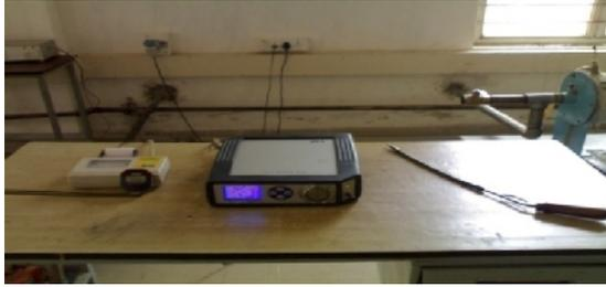
Fig. 3. Five Gas Exhaust Analyzer (AVI) with Probe
