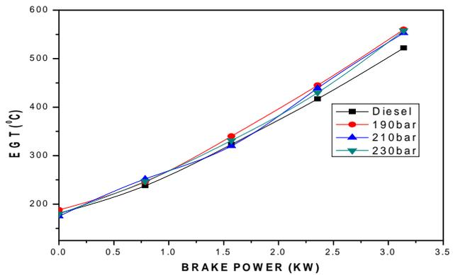
Fig. 7. Variation of EGT with Brake Power
