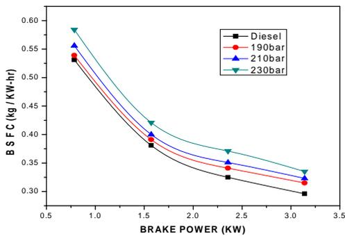
Fig. 4. Variation of BSFC with Brake Power
