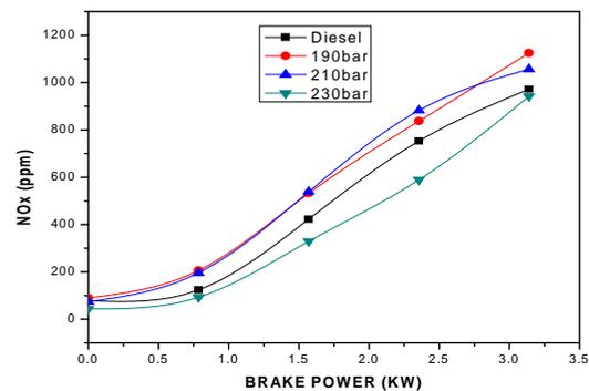
**Fig. 11.** Variation of NO<sub>x</sub> with Brake Power
