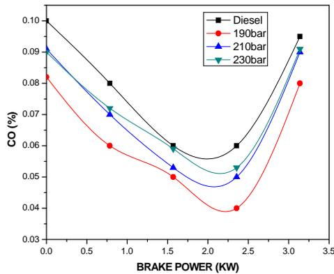
**Fig. 8.** Variation of CO with Brake Power.
