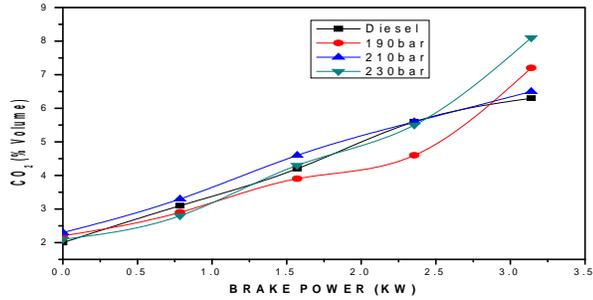
**Fig. 9.** Variation of CO<sub>2</sub> with Brake Power
