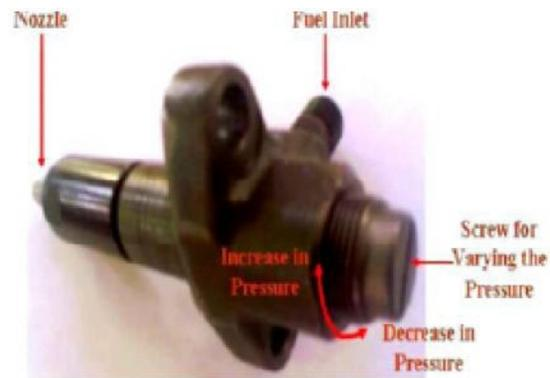
**Fig. 2.** Fuel Injector.
