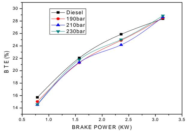
Fig. 6. Variation of BTE with Brake Power
