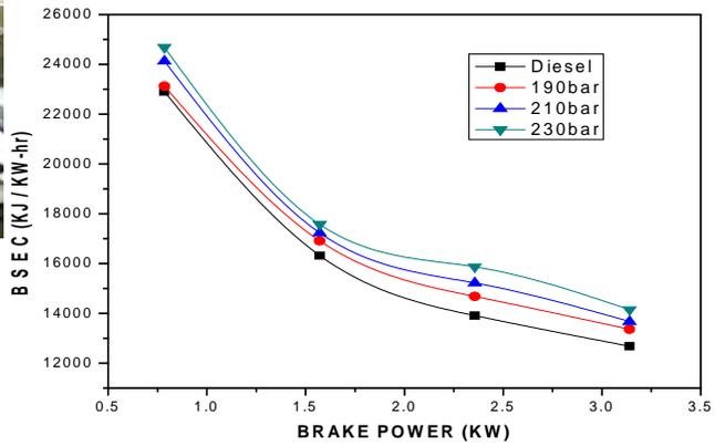
Fig. 5. Variation of BSEC with Brake Power
