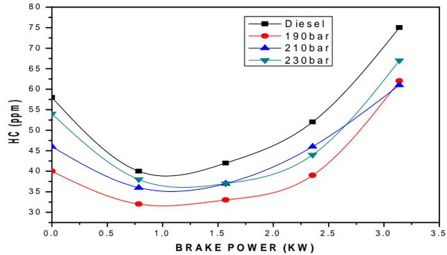
**Fig. 10.** Variation of HC with Brake Power
