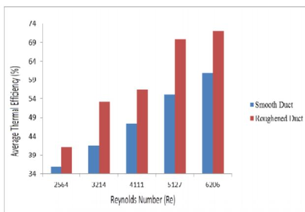
**Fig. 1.** Average thermal efficiency v/s Reynolds number between smooth and roughened duct.
