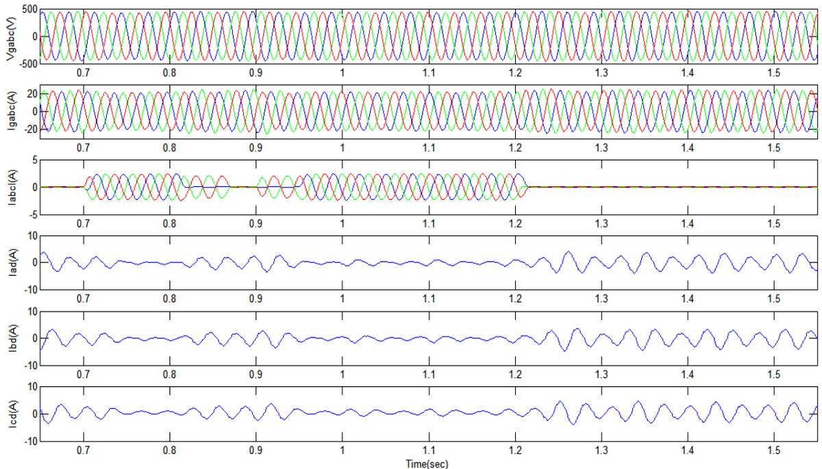
**Fig. 2.** Simulated transient waveforms of voltage generated by three-phase GIAG ( $V_{gabc}$ ), three-phase GIAG currents ( $I_{gabc}$ ), three-phase resistive load currents ( $I_{abcl}$ ), per-phase DLC currents ( $I_{ad}$ ,  $I_{bd}$ ,  $I_{cd}$ ).
