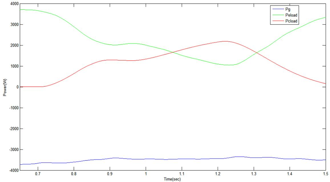
**Fig. 4.** Variation of power generated by GIAG ( $P_{gen}$ ), consumer power ( $P_{clload}$ ) and electronic load power ( $P_{eload}$ ).
