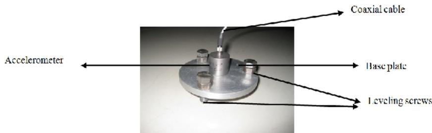
Fig. 1. Piezoelectric sensor with base plate.
