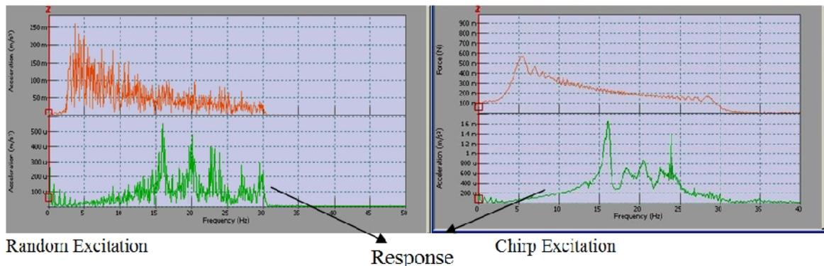
Fig. 2. Comparison of Random and Chirp excitation force spectrums.
