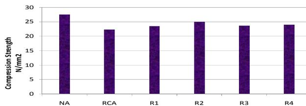
It is observed from the Fig above, compared to natural aggregate concrete; the compressive strength of recycled aggregate was decreased by 18.76%. The recycled aggregate treated with water has increased 4.93%, nitric acid by 11.88%, sulphuric acid increased
