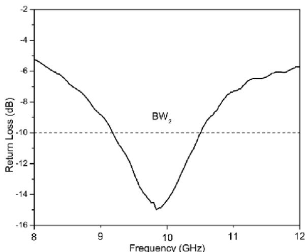
**Fig. 5.** Variation of return loss versus frequency of CSQMA.
