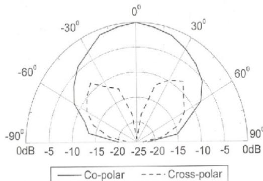
**Fig. 8.** Radiation pattern of CSQMA measured at 9.91 GHz.
