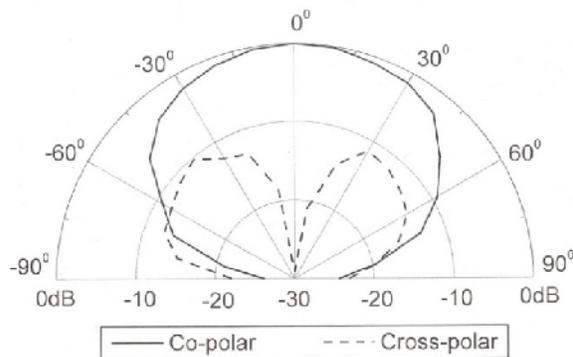
**Fig. 7.** Radiation pattern of conventional SQMA measured at 8.80 GHz.
