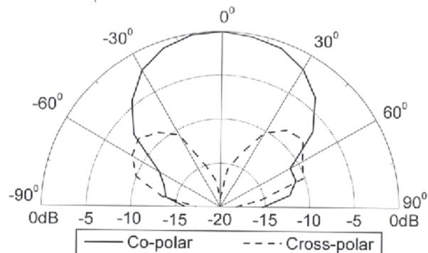
**Fig. 8.** Radiation pattern of SCSQMA measured at 9.91 GHz.
