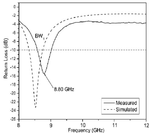
Fig. 4. Variation of return loss versus frequency of SMSA.
