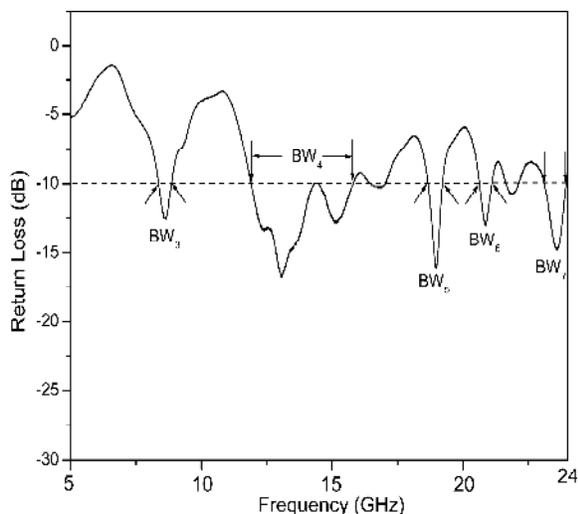
**Fig. 6.** Variation of return loss versus frequency of CSQMA.
