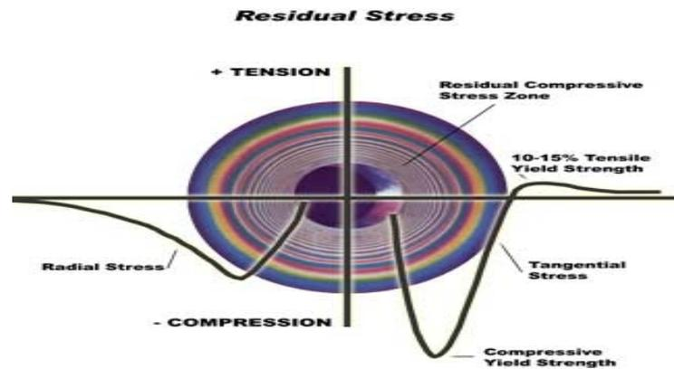
**Fig. 1.** Stress distribution around a cold expanded hole.
