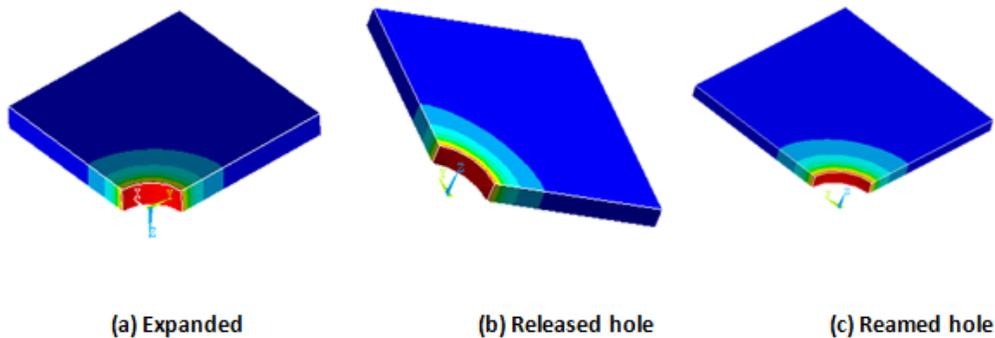
Fig. 5. FEM analysis of cold hole expansion in Al7075.
