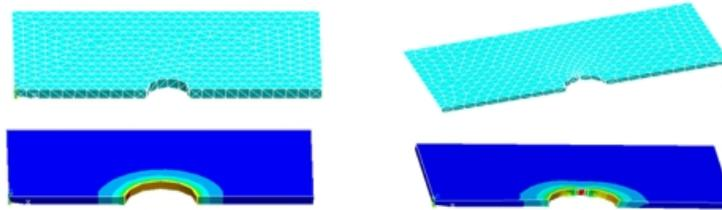
**Fig. 4.** (a) Cold hole, (b) Cold expansion of hole with a corner crack  $A/C = 1$ ,  $C/T = 0.6$ .
