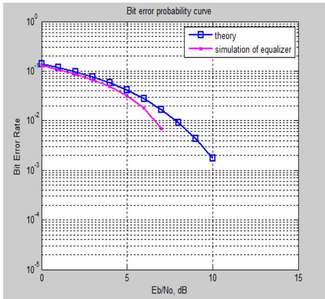
Fig. 2. BER plot of 2x2 MIMO Equalization.
