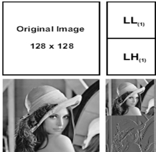
Fig. 3. Discrete wavelet transform (DWT) coding generating one and two levels of resolution [12].
