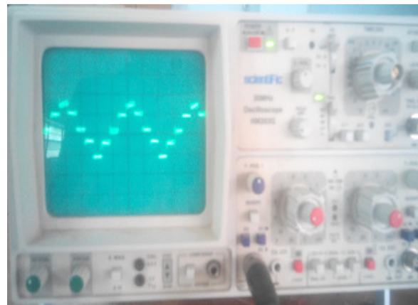
Fig. 5. Output five level staircase waveform.
