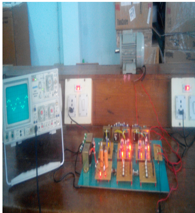
Fig. 4. Photograph of complete hardware setup.
