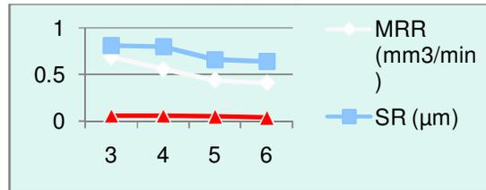
**Effect of Peak Current on Graphite PMEDM Process Characteristic**
