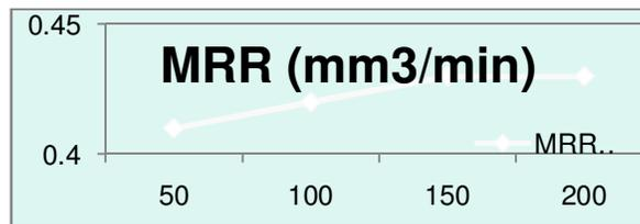
**Effect of Pulse off time on Chromium Powder on PMEDM Process**
