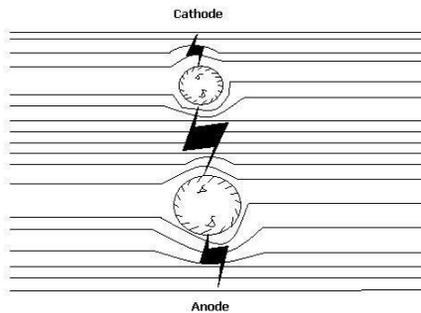
**Fig. 1.** Schematic Diagram of "Series Discharge" in PMEDM.
