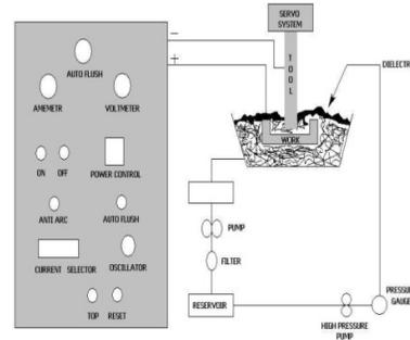
**Fig. 2.** Schematic Diagram of EDM Process.
