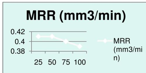
**Effect of Tool Electrode Lift time on Chromium Powder on PMEDM Process Characteristics.**
