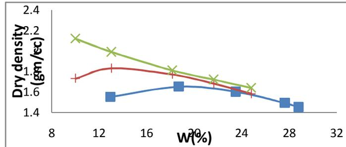
Fig. 2. Comparison of compaction Curves for both Light and Heavy Compaction of red soil
