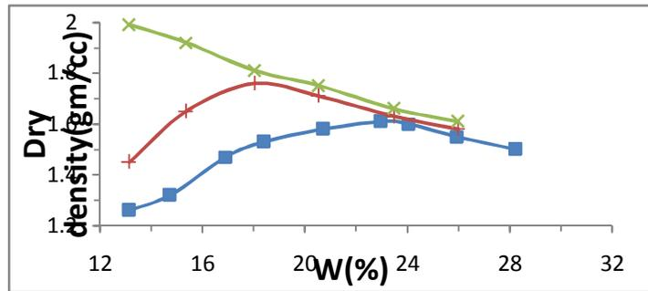
Fig. 1. Comparison of compaction Curves for both Light and Heavy Compaction of black cotton soil
