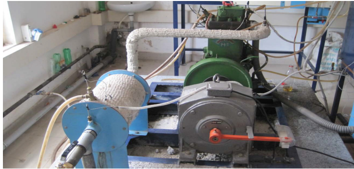
Fig. 4.9. Compression ignition engine set up used for experimental purpose.
