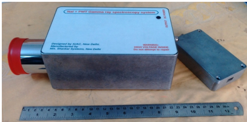
Fig. 3. Assembled view of spectroscopy unit.
