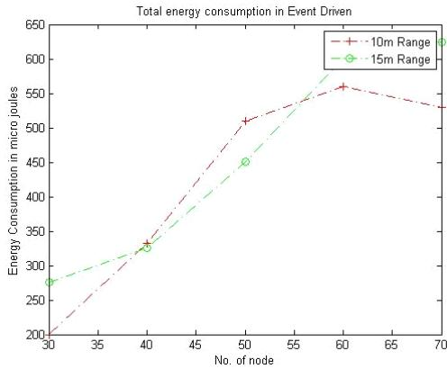
Energy consumption is the important parameter in the WSN network. Node have less energy as they are operated by battery power hence preserving the battery energy is the important concept. In this graph the nodes are considered in the x-axis and energy consumption is considered in the y-axis. Here in this case energy consumption is calculated for both event driven and user driven. The results shows that, as the communication range and number of nodes increases the energy consumption increase.
