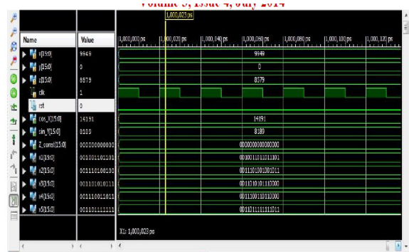
Fig. 2. Simulation waveform for 16 bit sine and cosine value.
