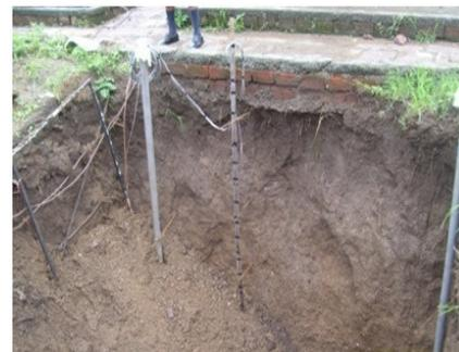
**Fig. 3.** Buried galvanized steel pipe of EAHE and thermocouples on a wooden strip.
