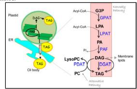
The current pathway involves three major spatially separated biochemical steps, i.e. plastidialfatty acid synthesis, acylation of fatty acids to glycerol, and deposition as oil bodies, the sub-cellular compartment destined for oil storage.
