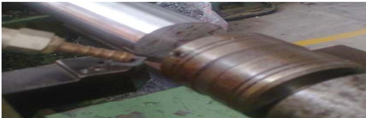
Fig. 1(b) Tool holder and coolant delivery nozzles.
