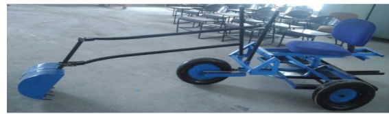
Fig. 8. Overall fabricated earth digger machine.
