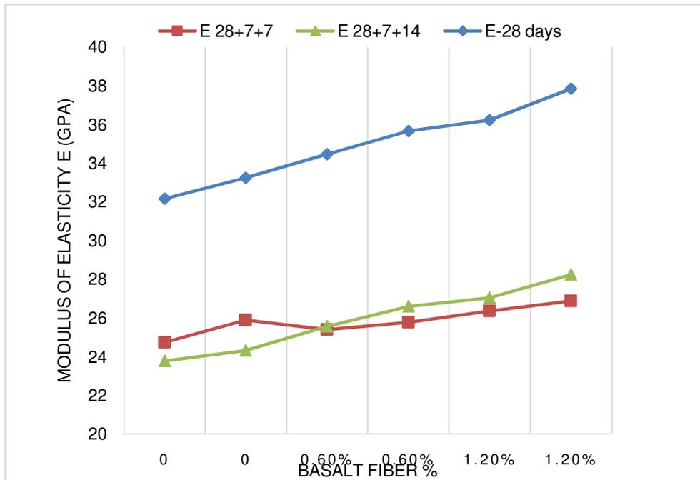
Fig. 2. The effect of basalt Fiber percentage and saltwater on the modulus of elasticity of LECA.
