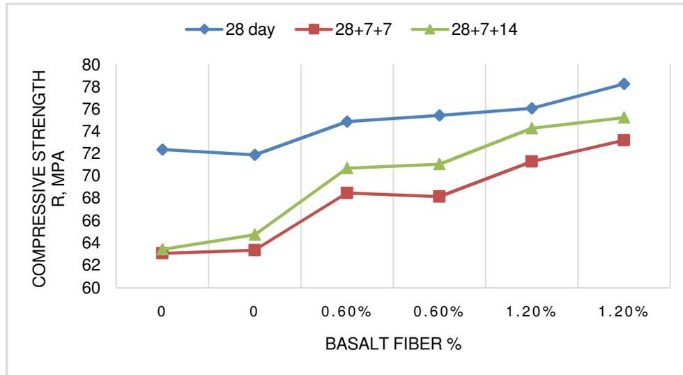
Fig. 1. The effect of basalt Fiber percentage and saltwater on compressive strength of LECA.
