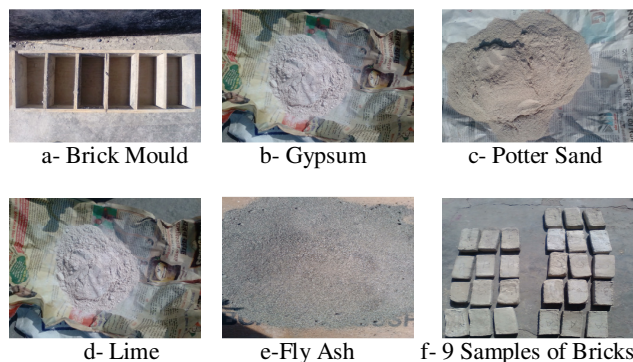
Figure 1: Different Material Composition used in Manufacturing of Fly Ash Bricks Pictures with Varying Samples and Mould.
