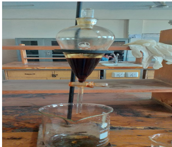
Fig. 1. Separating funnel for fractionation of S. fruticosa .
