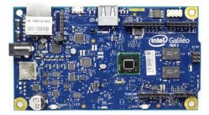
Fig. 15. Intel Galileo Gen 2 development board [35].
