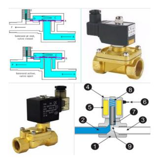
The solenoid valve drive unit controls the opening and closing of the solenoid valve which controls the flow gas from the supply to the point where the gas is being used. The solenoid valve drive receives signal from
