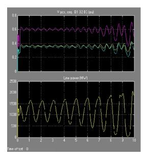
Fig. 9. Line power and bus voltage of without STATCOM.
