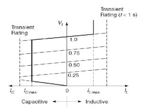
Fig. 3. The V-I characteristic of the STATCOM.
