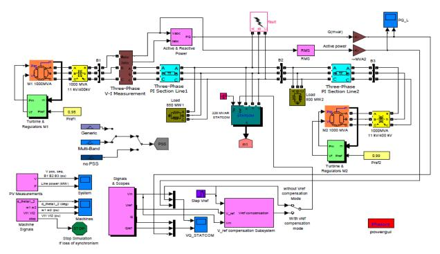
Fig. 6. MATLAB experiment model for transient stability test system.
