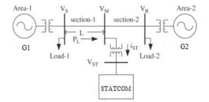
Fig. 5. Single line diagram infinite bus with fault.
