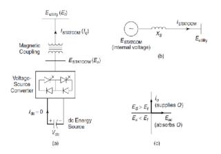
**Fig. 2.** The STATCOM principle diagram: (a) a power circuit; (b) an equivalent circuit; and (c) a power exchange from the ac system.
