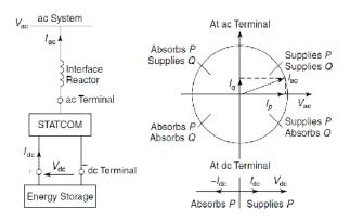
Fig. 4. The power exchange between the STATCOM and the ac system.
