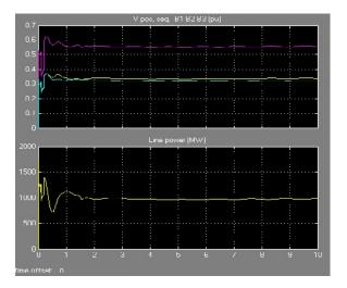
Fig. 10. Line power and bus voltage of with STATCOM.
