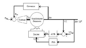
Fig. 1. Generation unit diagram.
