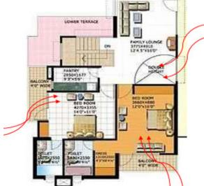
Fig. 22. Natural ventilation strategy in Purvanchal Height. (Source: Field Work, 2020).
