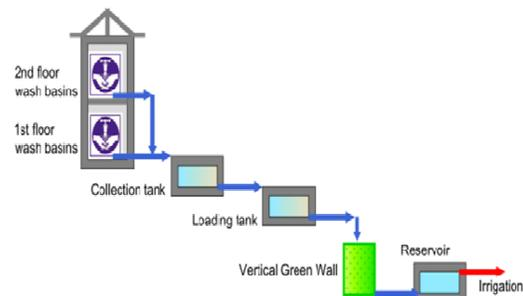
The inflow from the collection tank is stored in two intermittent loading tanks of 100Litre capacity each whose outflows are controlled by a timer based solenoid valve. The feeding of the treatment unit happens through hourly flush of 10Litre of greywater. The discharge is directly allowed to flow into the garden next to the walls.
