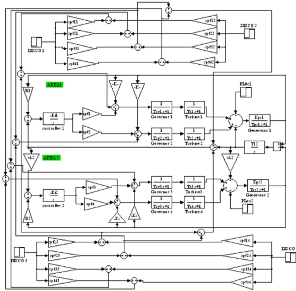
Fig. 2. MATLAB simulation model of two-area thermal system in deregulated environment.
