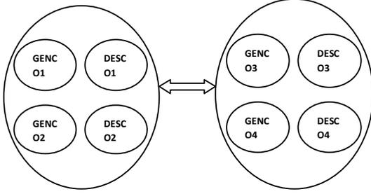
**Fig. 1.** The configuration of two-area interconnected power system in deregulated environment.
