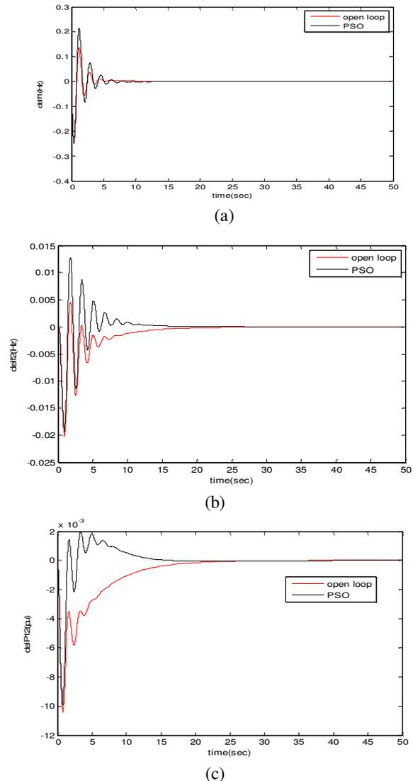
**Fig. 3.** (a) Frequency response of area 1. (b) Frequency response of area 2. (c) Deviation of tie-line power.
