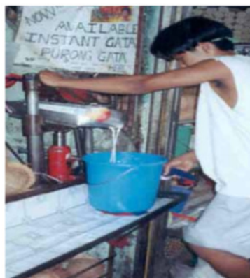
Fig. 5. Extraction of coconut milk using a manual hydraulic jack [17].
