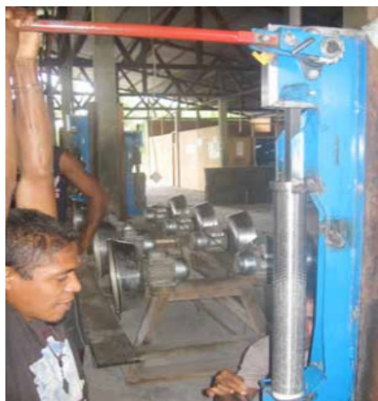
Fig. 11. Manual pressing of sapal [17].
