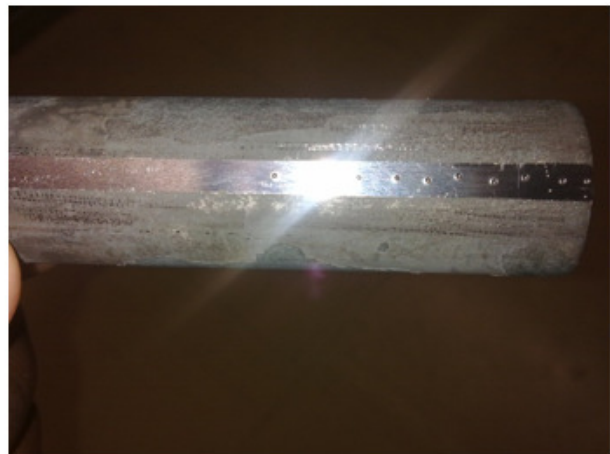
Fig. 7. Decarburized samples before and after indentation.
