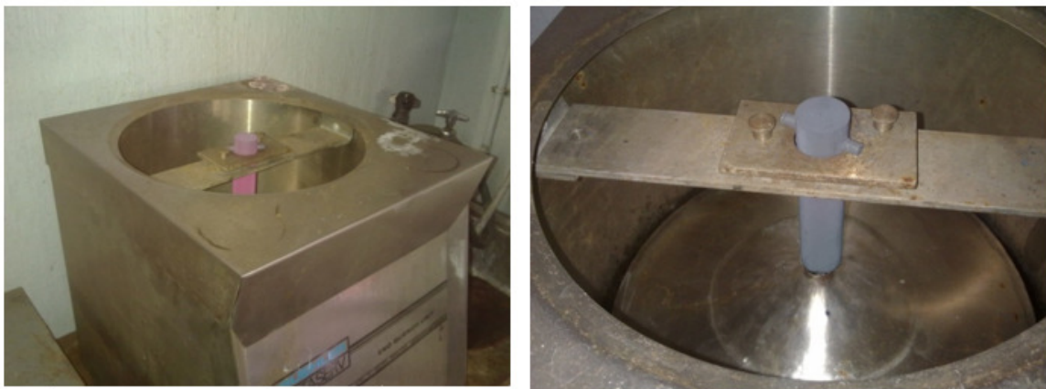
Fig. 6. (a) Jominy end-quench technique, (b) rapidly cooled steel sample by quenching.
