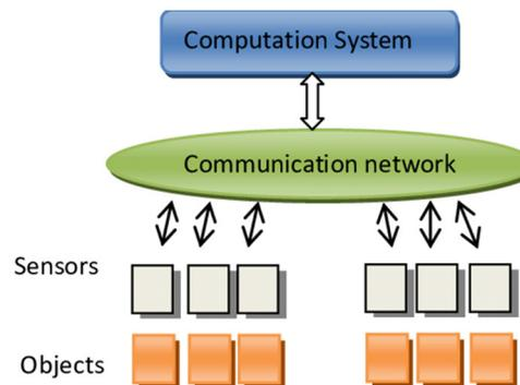
Fig. 1. Basic IoT Architecture
