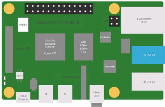
Fig. 6. Raspberry Pi Architecture.
