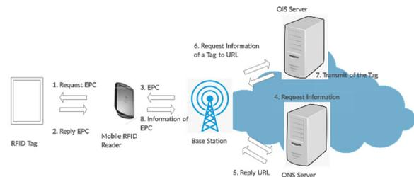
**Fig. 5.** Mobile RFID Network Architecture Overview [2].
