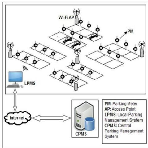
**Fig. 3.** E-Parking System [Smart Parking System Based On Internet of Things: A Review].
