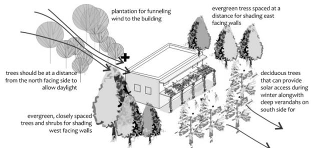
**Fig. 5.** Use of Vegetation for Shading and Ventilation in a Building.
