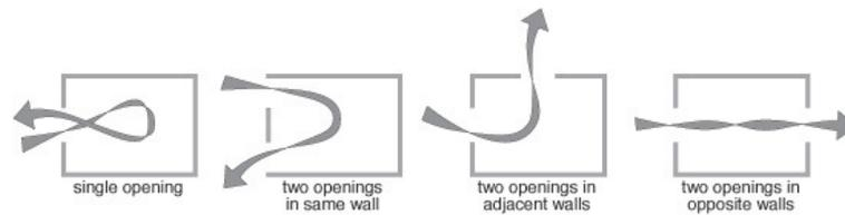
**Fig. 6.** Window opening types for maximum air ventilation in buildings
