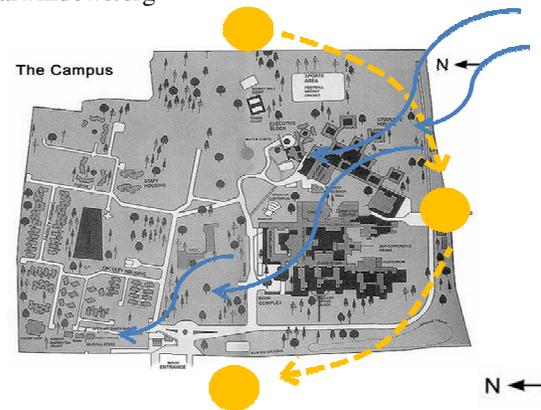
**Fig. 6.** The sun path and wind movement in the campus. Most buildings are oriented in the N-S direction (Source: Self).
