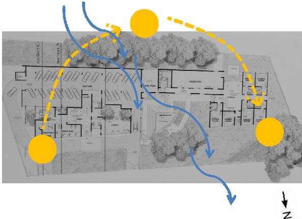
**Fig. 9.** The sun path and wind movement of the building.
