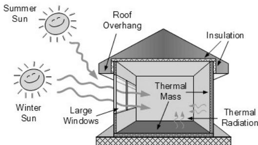
**Fig. 4.** Design using Thermal Mass combined effectively with other strategies.
