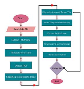
Fig. 13. IR image processing Algorithm.
