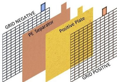
Fig. 1. Lead acid Battery with, negative grids, PE separator, Positive plate and positive.
