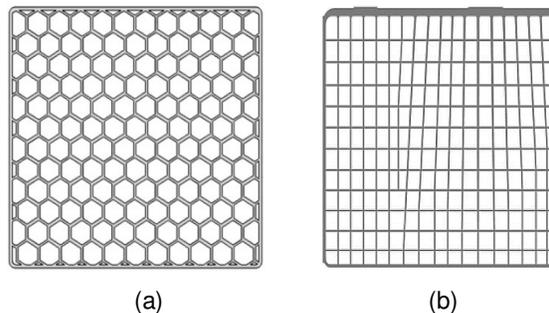
Fig. 2. Grid structure design as (a) Hexagonal and (b) Rectangular.
