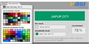
**Fig. 10.** Measure level of LRV contrast between text and background for existing signage (ASI).
