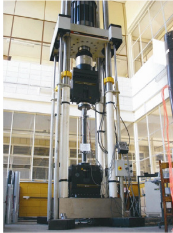
Fig. 1. Setup of experimental test of slender column [13].
