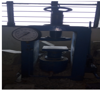
Fig. 14. Compressive Strength Testing Machine with 1000N/mm Pressure gauge capacity.
