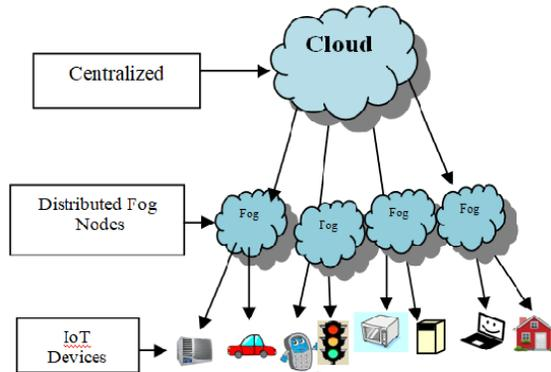
Fig. 1. Architecture of Fog Computing.
