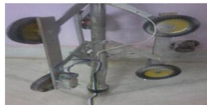
**Fig. 6.** Wheeled leg mechanism for robot.
