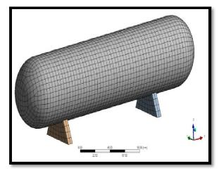
Fig. 1. Meshed Pressure vessel.
