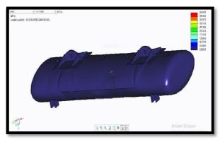
Fig. 6. Analysis of mild steel based pressure vessel.
