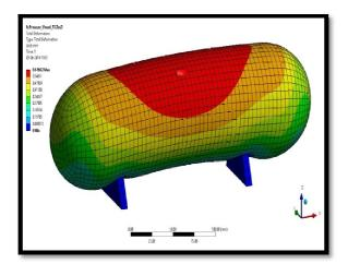
Fig. 2. Total deformation for 0% Al6082 alloy.
