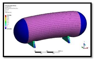
Fig. 5. Equivalent stress for Al6082/10% ZrO<sub>2</sub> AMCs.
